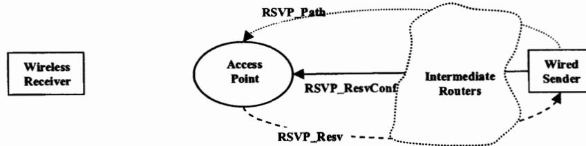
Figure 4. End-to-end reservation setup procedure of downlink flows
