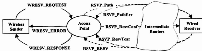
Figure 5. End-to-end reservation setup procedure of uplink flows
